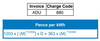
where **D** is the direct distance from the site or non-National Grid NTS pipeline to the elected terminal in km and **M** is Maximum NTS Exit Point Offtake Rate (MNEPOR) converted into kWh/day at the site. Note that ^ means "to the power of ..."
